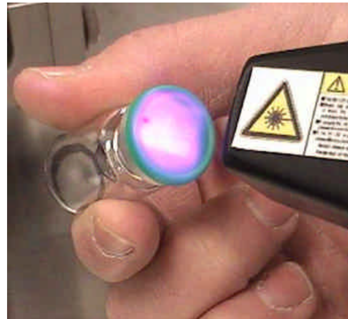
Pharmaceutical Vial with InData UV Scanner
